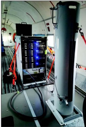
*UWBRAD instrument installed in the DC-3T aircraft. The cylinder in the foreground is the deployable 'periscope' antenna, and the instrument electronics are housed in the rack in the background. Image credit: Ohio State University.*
