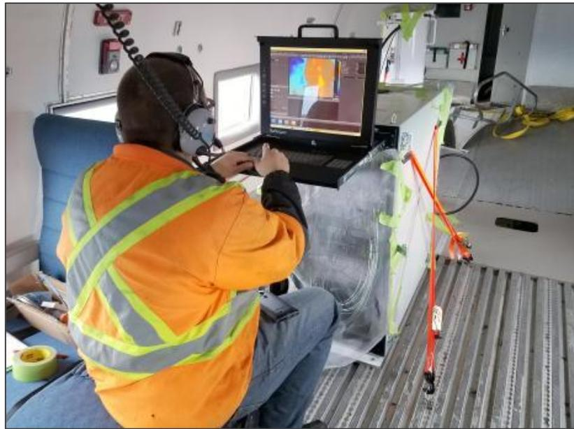
No methods currently exist for remotely sensing ice sheet internal temperatures; presently, the only measured information is obtained from a small number of deep ice core sites. As an airborne instrument, UWBRAD could obtain this type of data over wide areas. The airborne tests provided approximately 10 hours of the first ultrawideband microwave radiometer measurements of geophysical scenes including ice sheets. The UWBRAD project team intends to conduct additional test flights.
